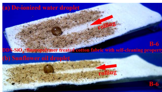
Figure 10. Image showing self-cleaning property of DDS-SiO 2 /fluoropolymer treated cotton fabric. [Color figure can be viewed in the online issue, which is available at wileyonlinelibrary.com .]
